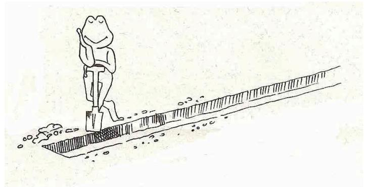
2. Dig a hole 95cm deep every 1.5m and sink the 4x4 posts. Secure the posts by hammering them down and surrounding them with soil. Make sure the soil around the posts is compact and the posts are sturdy.
